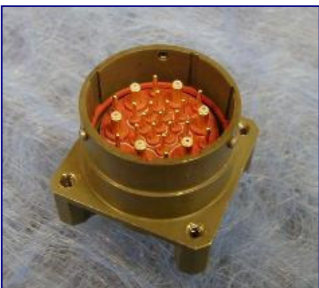
M26482 Receptacle with custom flange and built in helicoils for positioning PWB from the panel.
