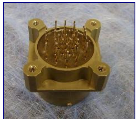
M26482 Receptacle with custom flange and built in helicoils for positioning PWB from the panel.
